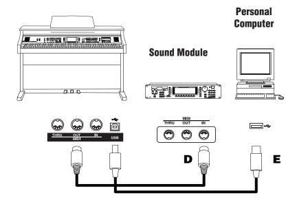
In order for the CP and your computer to properly communicate over this USB cable, you first need to set the MIDI-USB switch located next to the MIDI jacks to USB. Also your computer must have a USB driver installed. Please read the instruction on the next page for the details about the USB driver.
